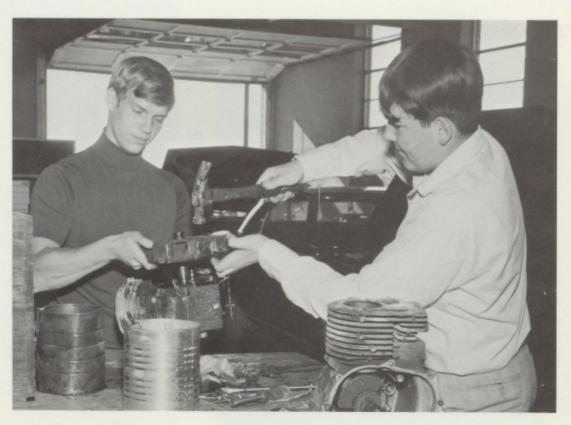
Lee Hollingsworth and Danny Piercy combine their knowledge of car engines with their physical strength to remove the case cover from the crank shaft.
