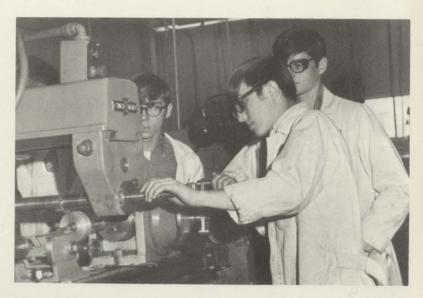
The cutting of a gear by horizontal milling machine is led by J. B. Spitzmesser.
