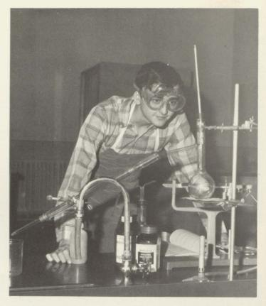
Fractional distillation of petroleum was measured by Chemist Ron Gill.
