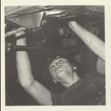
Front end rod bearings are put in by Greg Conwell.
