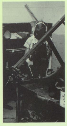
Using an arc welder, Roger Ice adds the finishing touches to the leg of a cattle table.
