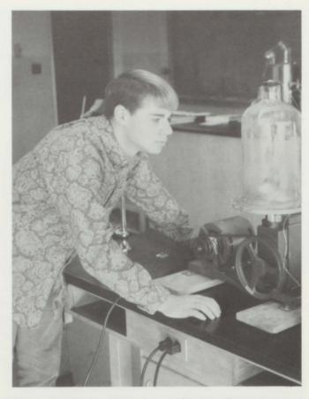
The non-conduction of sound in an electronically-created vacuum is carefully observed by Mike Ice.
