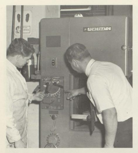
Mr. Rayshich explains the blade welder on the automatic bandsaw to Andy Daulton.
