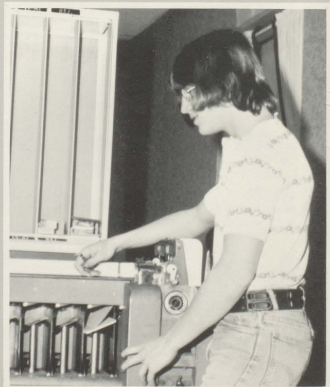
Kemmon Jones runs the punched data cards through a sorting machine in Computer Science.
