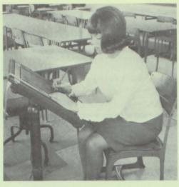
The mimeoscope, an illuminated drawing board, is used for preparing pictures in Gazette.
