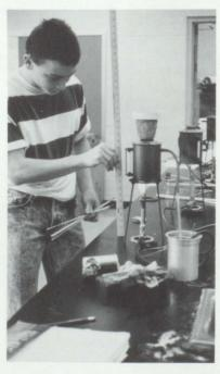
Pat Brown, 12, measures the specific heat of lead shot in boiling water. (M.A.)
